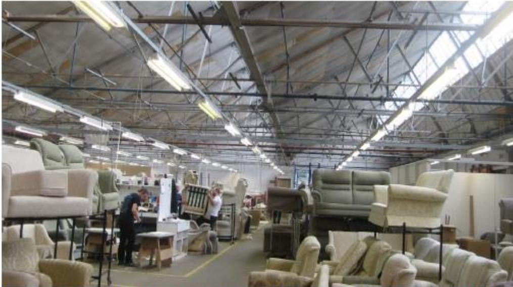
Interior of Vale factory. Note the wide span of the north-light roof structure and the thin structural members.
