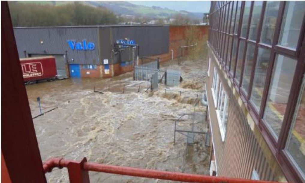
Boxing Day 2015 flood, looking upstream from Unit 2 Greenhill Ind Est. Note the effect of the bridge on flood levels and the depth of flooding in the downstream yard; the upstream end of the factory was under around 1.2m of floodwater. Also note fences & gates blocking overtopping flow.
